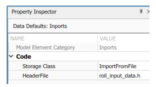
4 To see how the extern declarations in external header file roll\_input\_data.h name the input variables, in the MATLAB Command Window, open roll\_input\_data.h located in your current working folder.
