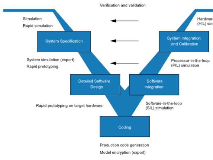
Depending on your application and its role in the process, you might focus on one or more of the steps called out in the V-model or repeat steps at several stages of the V-model. Code generation technology and related products provide tooling that you can apply to the V-model for system development. For more information about how you can apply MathWorks code generation technology and related products to the V-model process, see:
