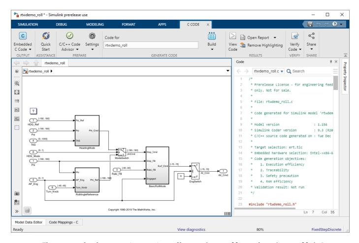
The generated code appears in two primary files: rtwdemo\_roll.c and rtwdemo\_roll.h. In your MATLAB current folder, the rtwdemo\_roll\_ert\_rtw folder contains these primary files.
