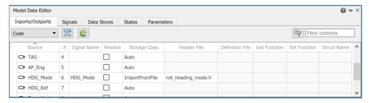
Based on these settings, the code generator imports the declaration for external variable HDG\_Mode from header file roll\_heading\_mode.h.
