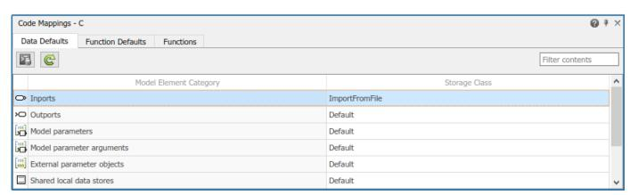
With this setting, the generated code does not define global variables that represent the inport data. Instead, a #include statement includes a header file that declares the input variables. You specify the name of the header file with the Property Inspector.
